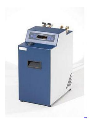
This picture shows a water-cooled version of a cooling unit. Thanks to its relatively small dimensions it can be easily positioned inside a laboratory cabinet or similarly confined space. Since the unit releases very little heat into the surrounding area, there is no need for ventilation of the installation location. The unit's performance is sufficient to supply up to three workstations with rotary evaporators.
